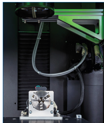
View of workspace including Z and rotary axis, fume extraction, and optical breadboard.
