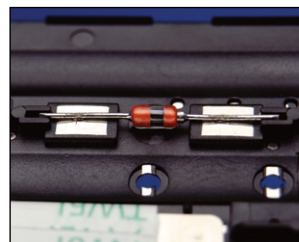
Welding components to leadframe
