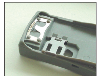
Heat stake thermode application mobile phone heat staking
