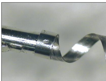
0.002 in (0.051 mm) thick platinum strip to platinum tube
