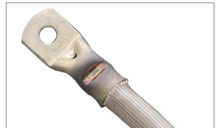
Hot crimping terminals to wire
