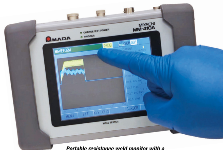
Portable resistance weld monitor with a touchscreen interface
