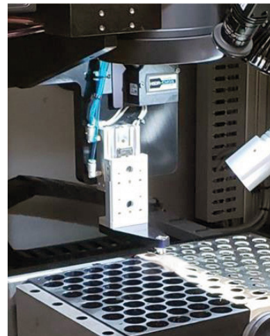
Fig. 6 - Laser welding system for battery pack manufacturing
