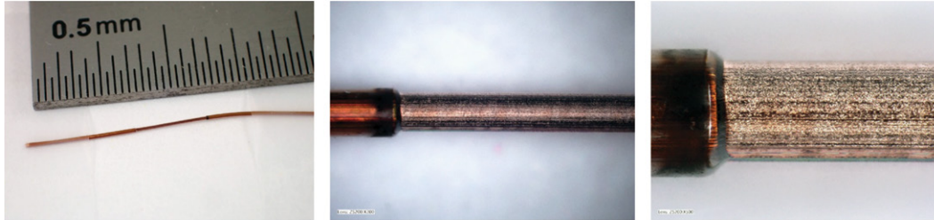
Figure 8: Example of ablated copper wire with a UV laser.
