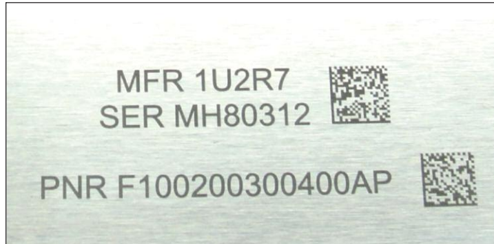
Figure 2 – Engraved mark in steel marked to UID MIL-STD 130 specifications
