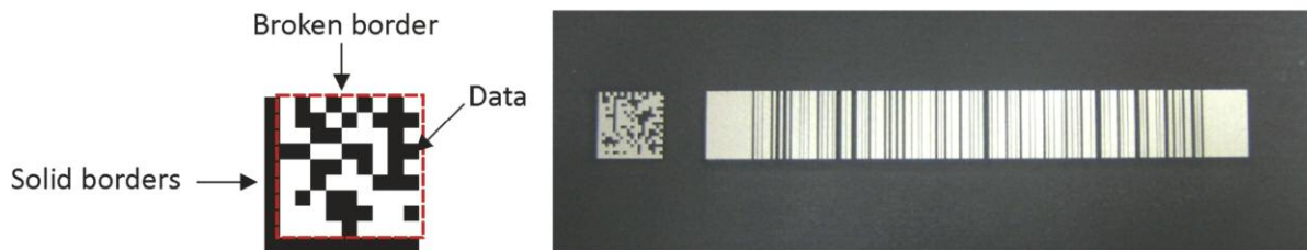
Figure 1 – Data matrix code compared to barcode
