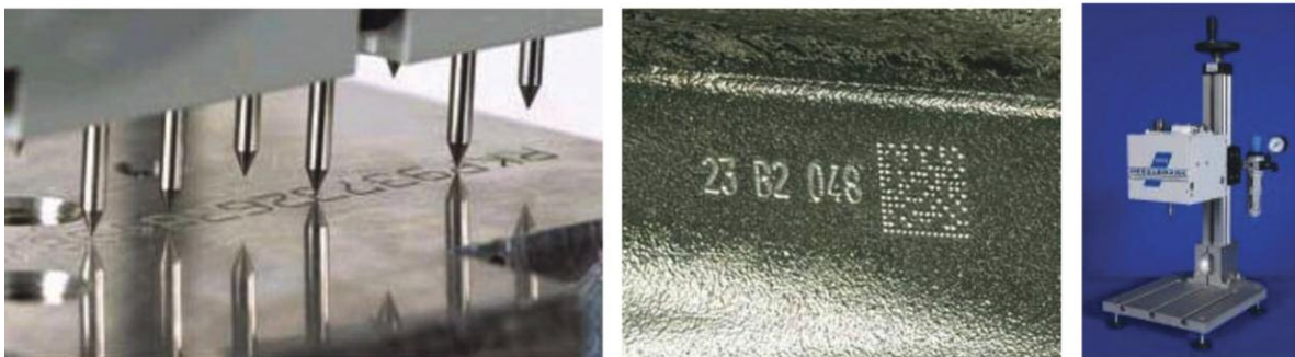
Figure 1 – Multiple stylus engraver, typical mark in aluminum and dot peen equipment
