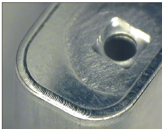
Figure 1 – Seam welding of aluminum cans
