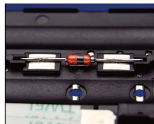
Welding components to leadframe
