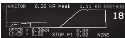
Monitor Screen – First pulse time automatically compensates for varying levels of oxides.
