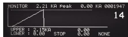
Monitor Screen – Shows weld current exceeding limit.
