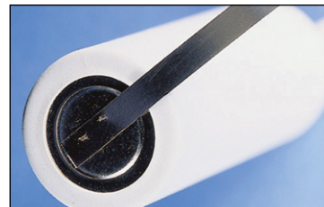
Tab to lithium-ion cell
