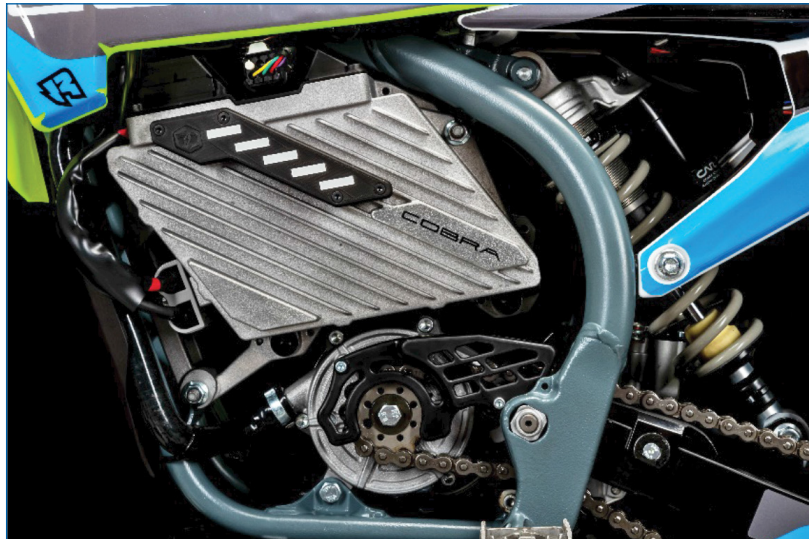
Figure 2 – Battery pack fits on either side of the motorcycle where the gas tank is usually located
