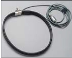
Toroidal coil MB-800P (ISO17657 compliant)
