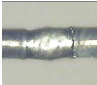
Guide wire welding
