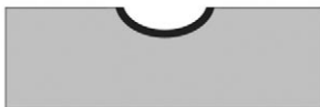
Material removal and surface melt, common in marks requiring lifetime readability in a demanding environment.
