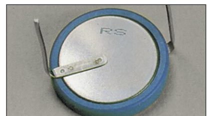
Battery tab welding
