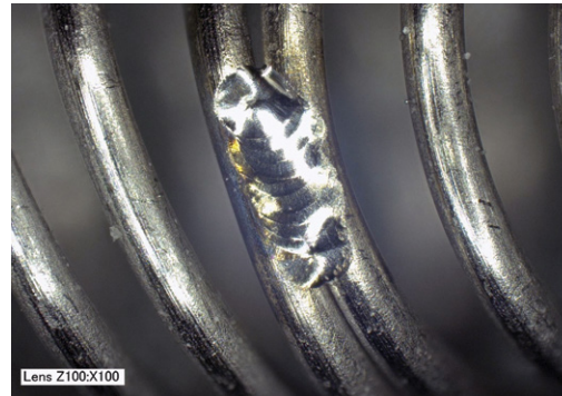
Side by side weld of canted coil wire.
