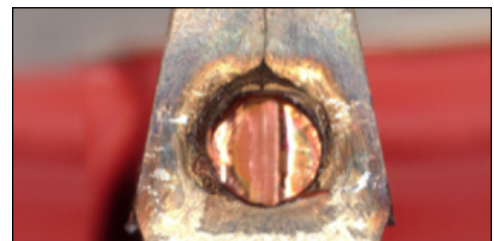
Fork weld for motor lead termination
