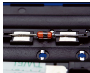
Welding components to leadframe
