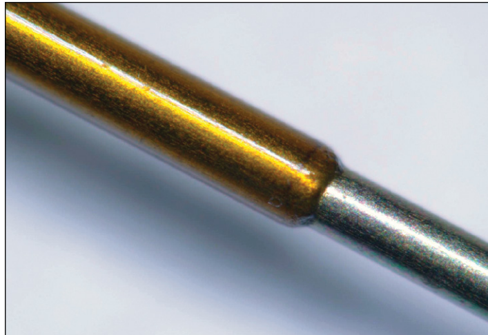
Figure 2 CO 2 laser stripping of polyimide wire insulation
