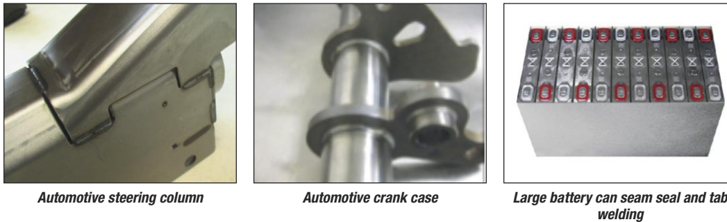
Figure 2 – Examples of high power CW laser welding
