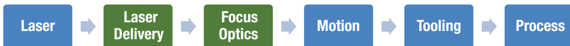
Figure 1: The essential components of a laser microwelding system. The laser delivery and focus optics bring the energy from the laser onto the workpiece.
