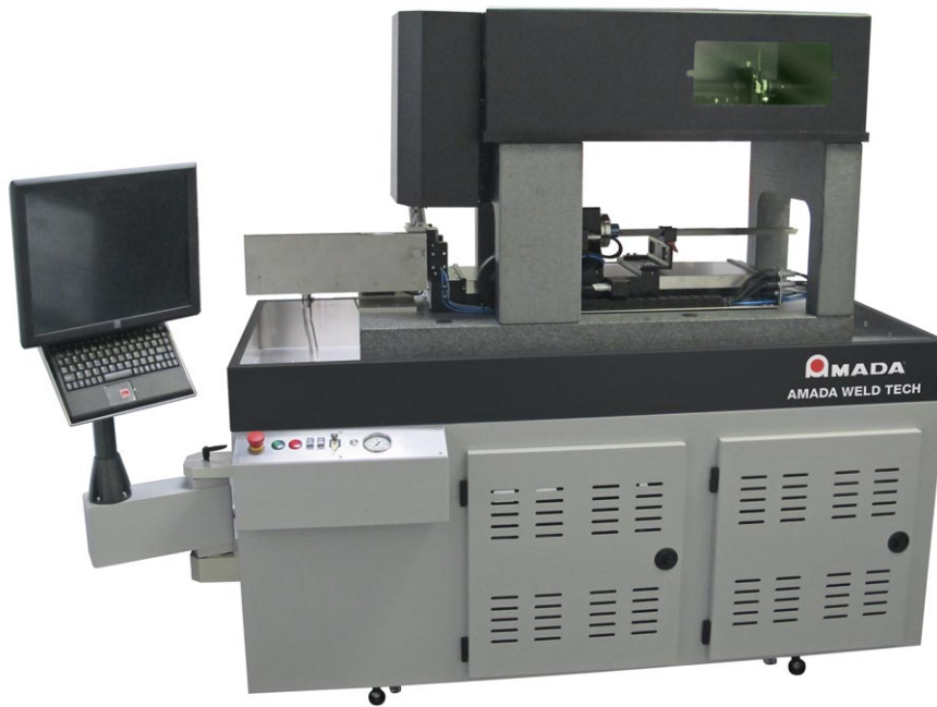
Figure 5 – Femtosecond stent and hypo tube cutter, covers off, showing Jenoptik laser
