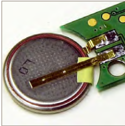
Solder reflow bonding battery tab to PCB
