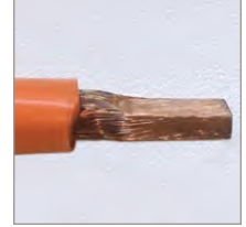
Stranded wire crimping and compacting
