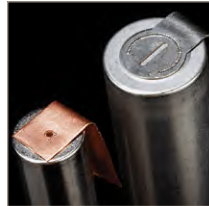
Battery tab welding
