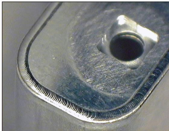
*Seam welding of aluminum battery housing by an Amada Miyachi America laser welding system*
