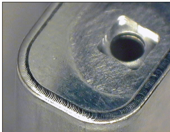
Seam welding of aluminum battery housing by an AMADA WELD TECH laser welding system
