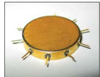
Seam welding circular electronic packaging
