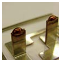
Micro TIG welding bus bars
