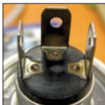
Micro TIG welding prongs
