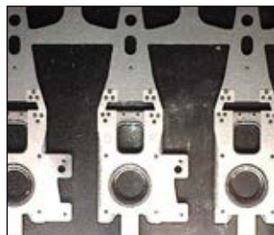
Laser spot welding disk drive arms
