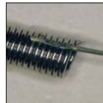
Spot welding wire to coil
