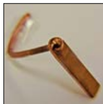
Micro TIG welding copper wire to bars
