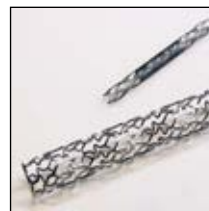
Laser cutting stents
