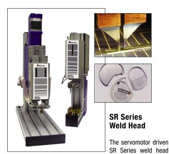
with overforce protection and soft-touch part clamping provides superior force control from 0.5-15 lb. with excellent follow-up. The SR Series, available in both opposed and parallel gap can store 32 motion control schedules for position and speed. The heads are ideal for automation and delicate or critical parts welding and work well with either the UB-500A or UB-1500A.
