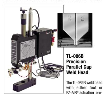
vides precision control for parallel gap welding applications from <0.001 inch (25 microns) to 0.005 inch (0.127 mm) in diameter or thickness. The force range of the TL-086B is 0.5 to 20 lbs. (2.2-89 N). EZ-AIR technology prevents overforce and guarantees force repeatability. The TL-086B is normally matched with the UB-500A or UB-1500A power supply.
