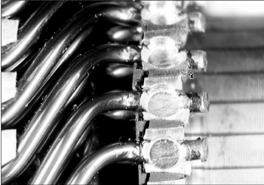
Minimized burn back using AC Inverter
