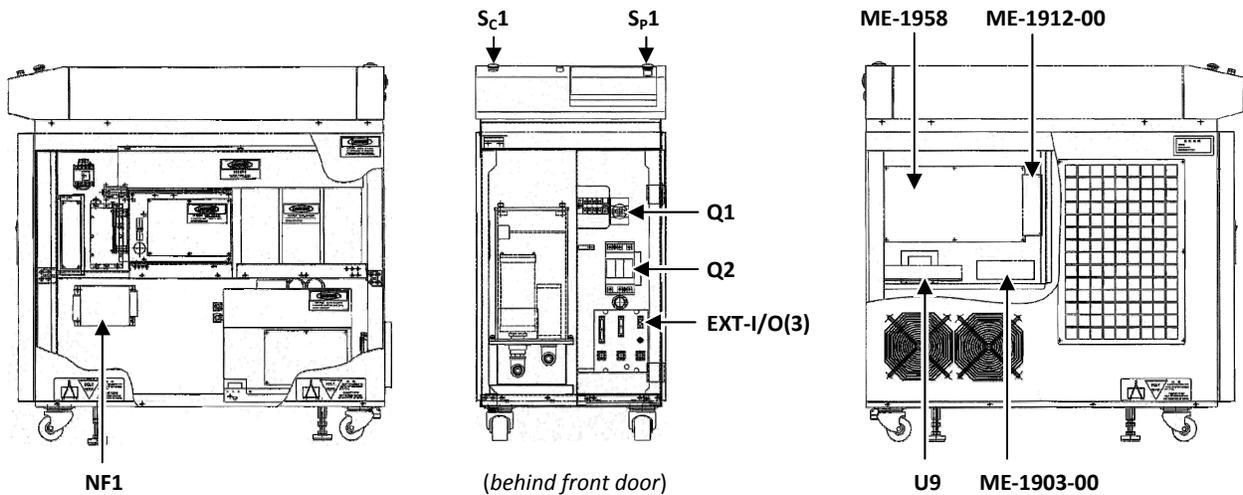
**LW50AE/70AE/150AE Component Locator**
