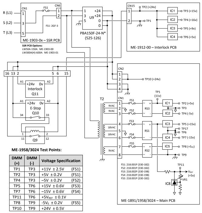
Note: +5V<sub>REF</sub> is adjusted by VR1 on Main PCB
