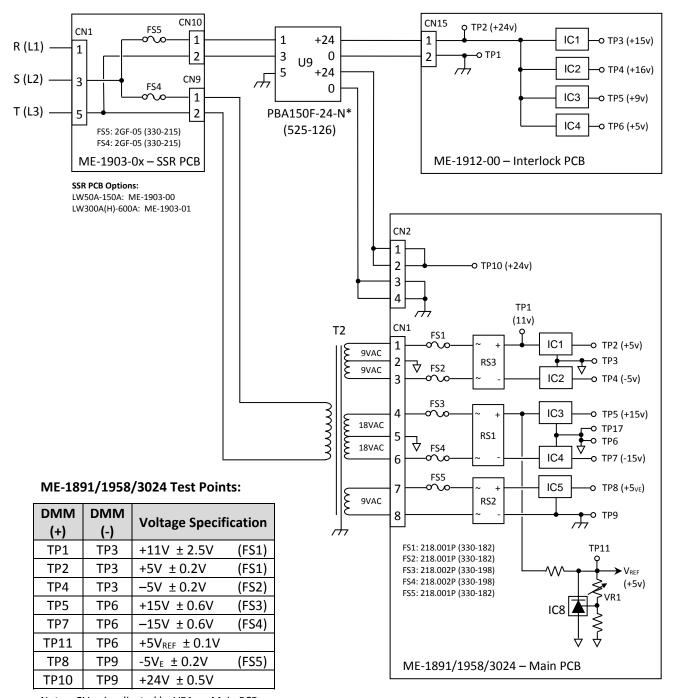
Note:  $+5V_{REF}$  is adjusted by VR1 on Main PCB
