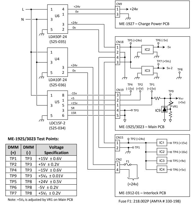
U4, U5 and U6 are mounted to the inside chassis wall behind the Main PCB and Interlock PCB.
