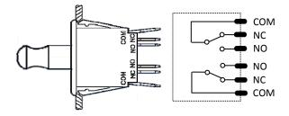
Note: In the schematics above, the connections shown are simplified (i.e. the actual wiring is more complicated than shown). When testing an individual switch, check the connections on the switch itself, then inspect the harness.
