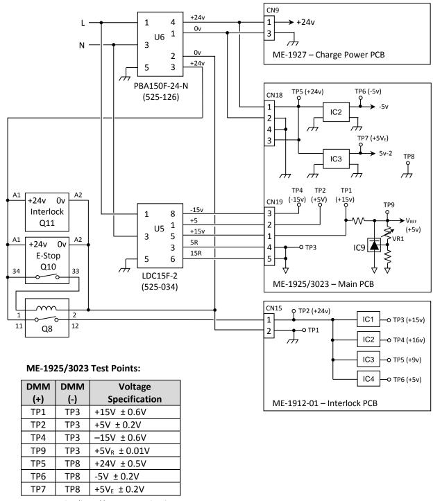
Note: +5V<sub>R</sub> is adjusted by VR1 on Main PCB
