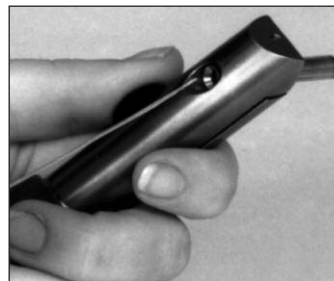
(1) Load stripped wire
