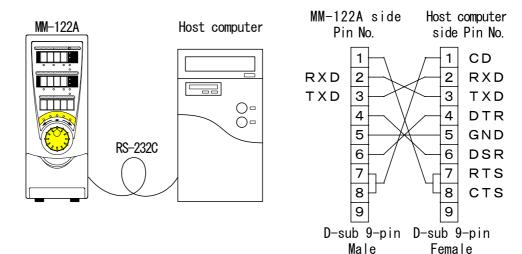
DTR and DSR are not used in **MM-122A**. Also, CTS is not checked at the start of sending.
