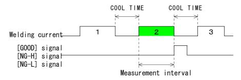
If the welding current doesn't reach the stage set in the pulsation measurement, the [NG+24V] signal and the [NG-H] signal are output.
