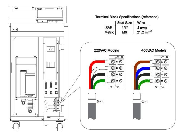
Note: The power cable shipped with the laser is terminated with ring terminals.
