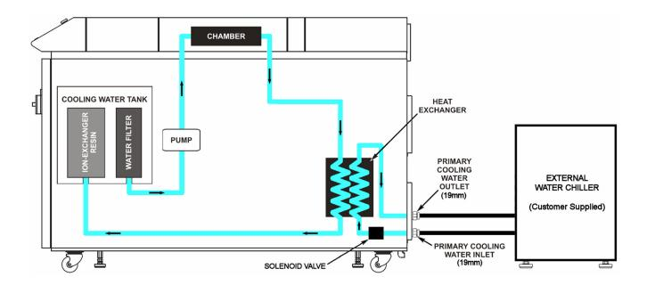
Temperature is maintained by allowing the primary cooling water to cycle through the laser. Once the secondary cooling water reaches a predefined temperature set-point, the *Solenoid Valve* is energized which allows the primary cooling water to flow through the *Heat Exchanger* (radiator). Once the secondary cooling water reaches the low temperature set-point, the Solenoid Valve is turned off. The primary cooling water supply should be connected to the hose barbs on the rear panel of the laser.
