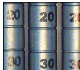
Passivation & corrosion resistant marking
