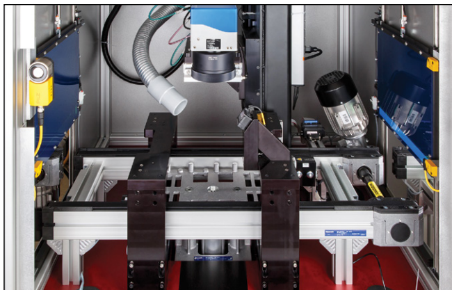
System work area with pallet lift to position parts in laser focus
