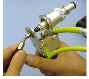
4. Inspect the fiber end for dirt or contamination. The fiber end will look similar to the following:
