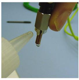
6. Blow air across the fiber end to remove the acetone and any loose dirt or particulates. Re-inspect the fiber end.
