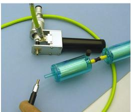
3. Connect each end of the fiber optic cable to the fiber optic end scope. Take care when inserting the fiber optic cable. Insert the cable at a slight angle to prevent the fiber end from getting scratched on the end face of the fiber optic end scope (as shown in the picture).
