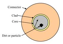
Note: You can only inspect one end of the cable at a time. To inspect the opposite end, reverse the cable to inspect.
