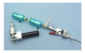
2. Blow air at an angle across each end of the fiber optic cable to remove any loose dirt or particulates.
