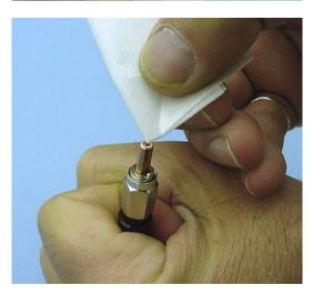
It is important to remember where the particulates are on the fiber end each time you make a cleaning pass. If the particulate appears in the same spot after numerous cleanings, then the fiber may be damaged. When the image in the fiber end scope appears clear and free of particulates, then the fiber end is "clean". If you can see any particulate in the fiber end scope *no matter how tiny*, it is considered dirty.
