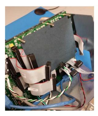
12. (Optional) Take the new LEC-2 card out of the anti-static bag. It is sometimes useful to write down the serial number and MAC address on a piece of tape and attaching it to the rear panel. WinLase recognizes these numbers and is a nice reference when verifying an installation.
