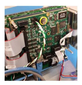
10. Loosen the 4 corner stand-offs with either a 3/16" or 4.5mm driver, just a little, then remove by hand.
