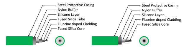
100μm and 300μm optical fibers
