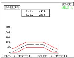
②As the screen shown in the left, when the welding is performed on the ENVELOPE screen, in addition to the measured current waveform, waveforms for monitor judgment are displayed in red, which are the upper limit which is 20 A higher than the measured current waveform and lower limit which is 20 A lower than the measured current waveform. When the measured current exceeds these red lines, it is judged as NG.
