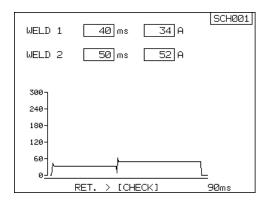
①When the CHECK key is pressed after welding, the screen shown in the left is displayed. Press the CHECK key again to return to the previous screen.
