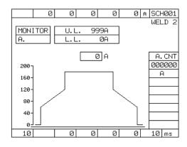
①Each time the SHIFT key is pressed, the first welding screen and the second welding screen are toggled.
