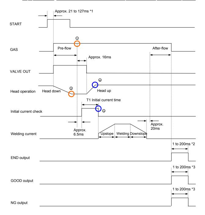
Note: Connect the VALVE OUT output signal (37 pins, D-Sub connector, 1: VALVE\_OUT\_COM, 2: VALVE\_OUT) to the solenoid valve input of the air-driven head or the head down/up input of the servo-driven head. To match with the head down/up time, distance between electrode and workpiece, production takt, etc, set pre-flow time, T1 time (initial current time), and P1 (initial current output value) to find optimum conditions.
