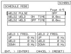
**WELD2 PULSE** : ON/OFF Turns on/off the pulse modulation for weld time in second welding.
