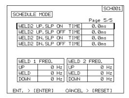
WELD2 UP.SLP ON TIME: 0.0 to 999.9ms Sets the ON time of pulse modulation in second welding upslope.
