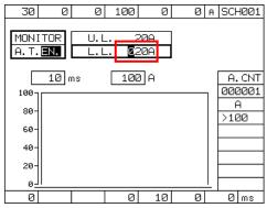
③Enter a value and press the LOWER key again or the ENTER key.
