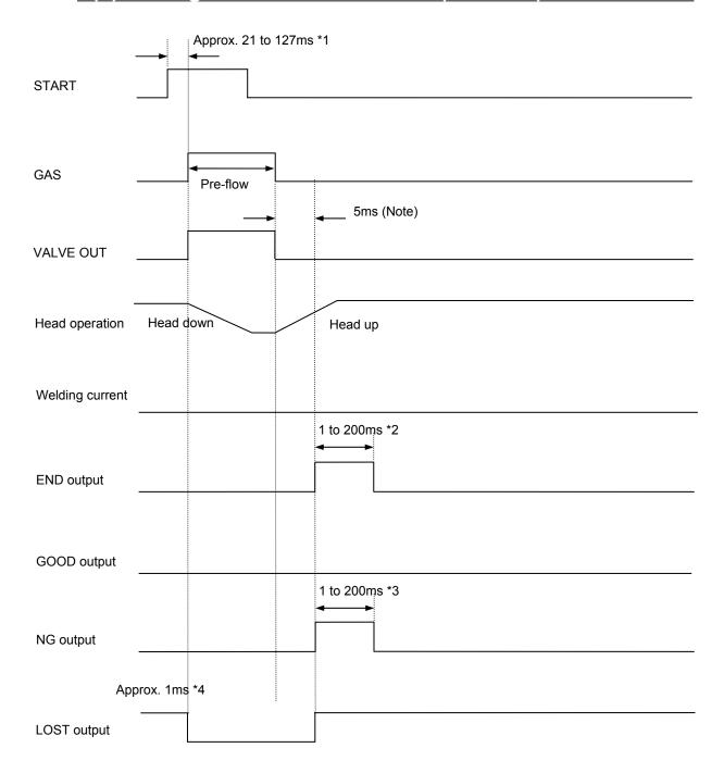
Note: In this interval, the initial current is checked.
