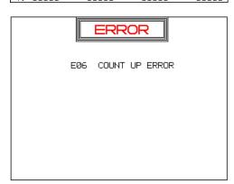
③When the start signal is input after the total count value becomes equal to the preset count value, the "COUNT UP ERROR" error screen is displayed, as shown in the left.
