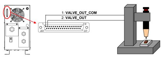
The VALVE\_OUT output signal (37 pins, D-Sub connector, 1: VALVE\_OUT\_COM, 2: VALVE\_OUT) on the rear of **MAWA-300A** is used. Connect the VALVE\_OUT output signal to the signal input for moving the air-driven head or the servo-driven head upward/downward.
