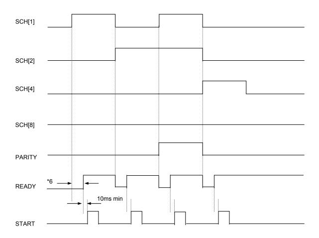
Note: The above timing chart shows the SCH# change from 1, 2, 3, to 4. Before turning on the START signal, set the SCH[1] to SCH[64] and PARITY. Then **confirm that the READY signal**, followed by the START signal turn-on.
