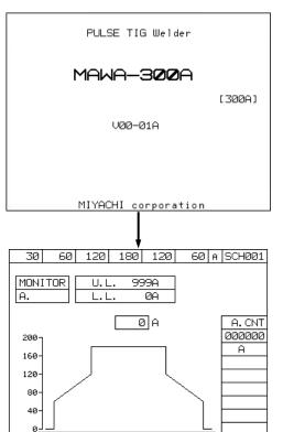
(1) The program display shows the model name and the ROM version for a few seconds, which is shown in the left, at right after turning the power on.
