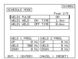
When times are set to ON TIME and OFF TIME and PULSE is set to ON, the frequency is displayed.
