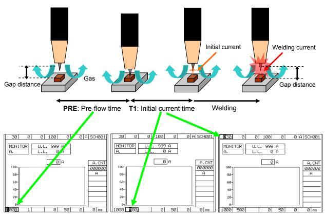
① **PRE**: Pre-flow time setting ② **T1**: Initial current time setting ③ **P1**: Initial current value setting Repeat adjustments of ①, ②, ③, and gap distance to find optimum conditions.
