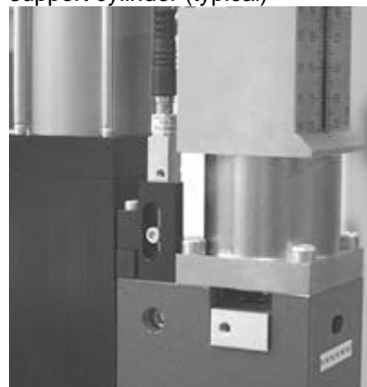
Illus. 21: F160 with scale housing and proximity switch ("Cushioned head")
