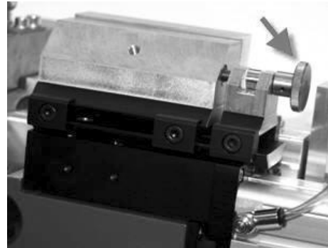
Illus. 24: Clamp and adjusting screw for the electrode distance (typical)
