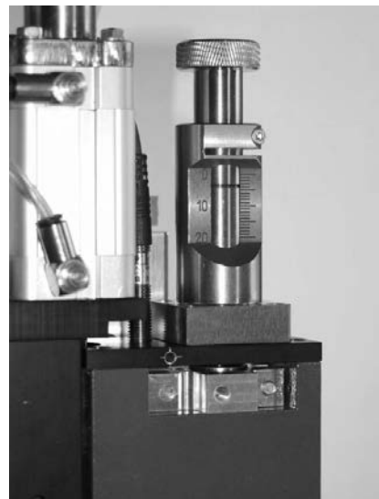
Illus. 29: F120 scale housing for setting the welding force (similar in principle to the F160)
