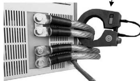
Illus. 12: Built-in flap toroid coil
