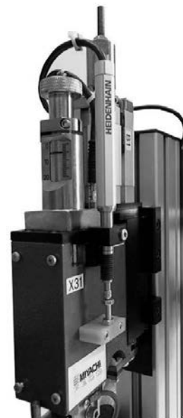
Illus. 14: Built-on, isolated displacement system
