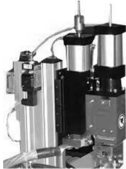
Illus. 3: Pneumatic connection of support cylinder (F160 in this case)
