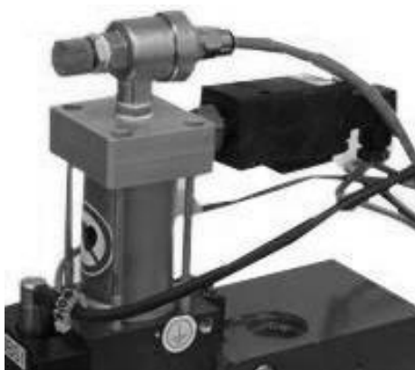
Illus. 1: Pneumatic connection of welding cylinder (typical) and pressure sensor for version with proportional valve control
