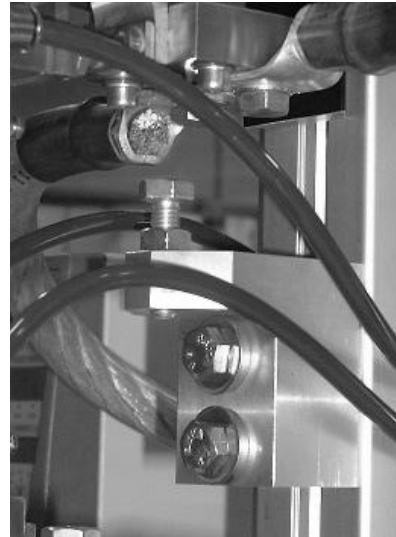
Illus. 19: Stop with locking nut - F160-M (typical)
