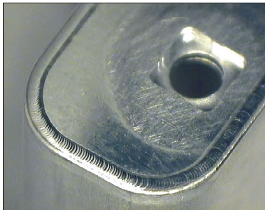
Figure 1 – Seam welding of aluminum cans
