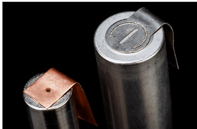
Figure 4 – Examples of laser welding conductive tabs
