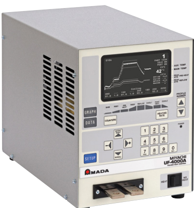
Power Supply delivers AC current to Thermode
