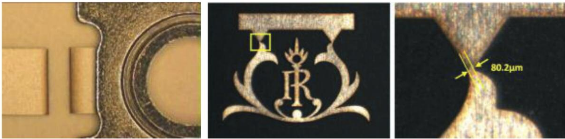
Figure 8 – Cut resolution and level of thermal heat input control
