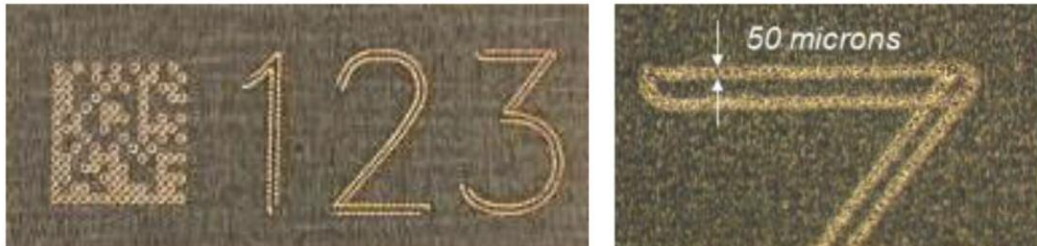
Figure 5 – Finer resolution and increased field size
