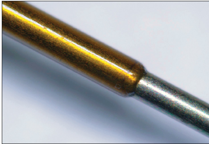
Figure 2 CO 2 laser stripping of polyimide wire insulation
