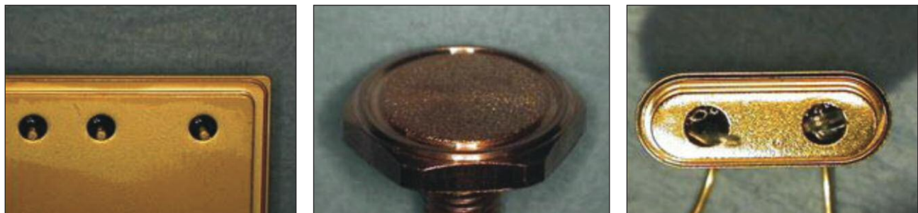
Figure 2 – Projections on the package header
