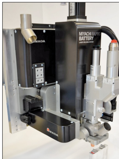
Figure 4 – Laser welding focus head with integrated tooling
